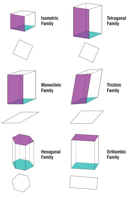
Please note: drawings underneath show the shape of the base of the crystals.
