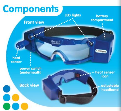
Your Thermo Goggles open up the invisible world of infra-red heat. Unlike night vision devices that rely on amplification of light, your heat-seeking goggles rely on detection of human and animal heat.
